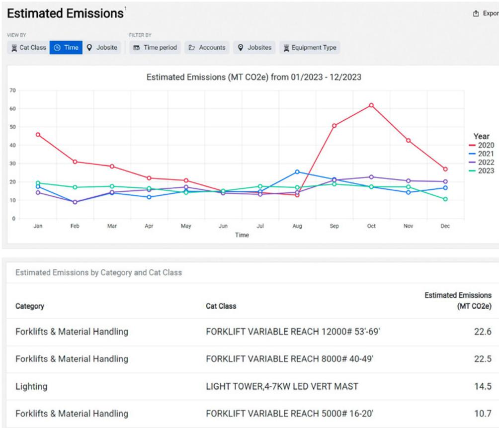
Portable generators may be the biggest GHG emission producers on one jobsite, while forklifts, telehandlers or excavators might be the biggest on others. Data unlocks the power to analyze which equipment to substitute with cleaner-burning alternatives.
